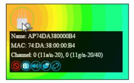
Click and drag an AP icon to move the icon around the zone map. The signal strength for each AP is displayed according to the "Signal" key in the menu on the right side:
