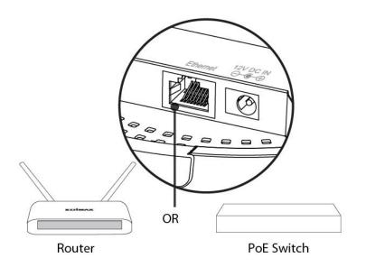
**3.** If you are using a router, then connect the power adapter to the access point's 12V DC port and plug the power adapter into a power supply.
