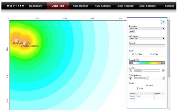
**Zone Plan** displays a customizable live map of Managed APs for a visual representation of your network coverage. Each AP icon can be moved around the map, and a background image can be uploaded for user-defined location profiles using **NMS Settings**  $\rightarrow$  **Zone Edit**. Options can be configured using the menu on the right and signal strength is displayed for each AP.
