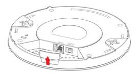
**2.**Connect a router or PoE switch to the access point's **LAN** port using an Ethernet cable.
